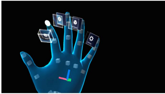
Top fingertip 1 - Hand tracking issues 2 - Hand fatigue holding hand above normal posture 3 - Issues pressing buttons with other fingers by accident due to limited space between fingers
